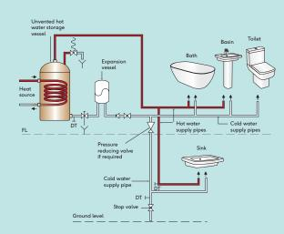
The unvented cylinder stores hot water at mains pressure, usually between 2 and 3 bar, allowing hot and cold water to be delivered at the same pressure. This means a power shower can be achieved without the need of a pump. All LP, MP and HP taps and fittings may be used.
