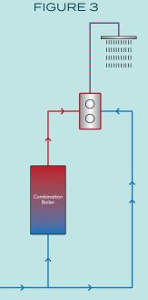
A combination boiler heats water on demand, and although it is fed by mains pressure this is regulated to the speed which the boiler can heat the water.
