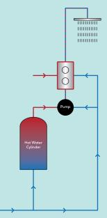
A pump assisted system will deliver water at high pressure and depending on the specifications of the pump fitted LP, MP and HP taps and fittings may be used.
