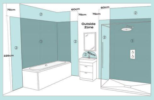
ZONE 0 – is inside the bath or shower. Any fitting used in this zone must be low voltage (max 12v) and be rated at least voltage (max 12v) and be rated at least IP67 (immersion proof) **BATHROOM REGULATIONS**
