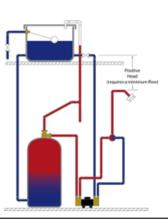
A 'Standard' peripheral pump allows water to run through its pump heads even when it's not running. The pump has a flow sensor that detects this flow to switch the pump on and boost water pressure and flow. The flow switch needs a flow due to gravity alone of at least 1 litre per minute to activate the pump.
